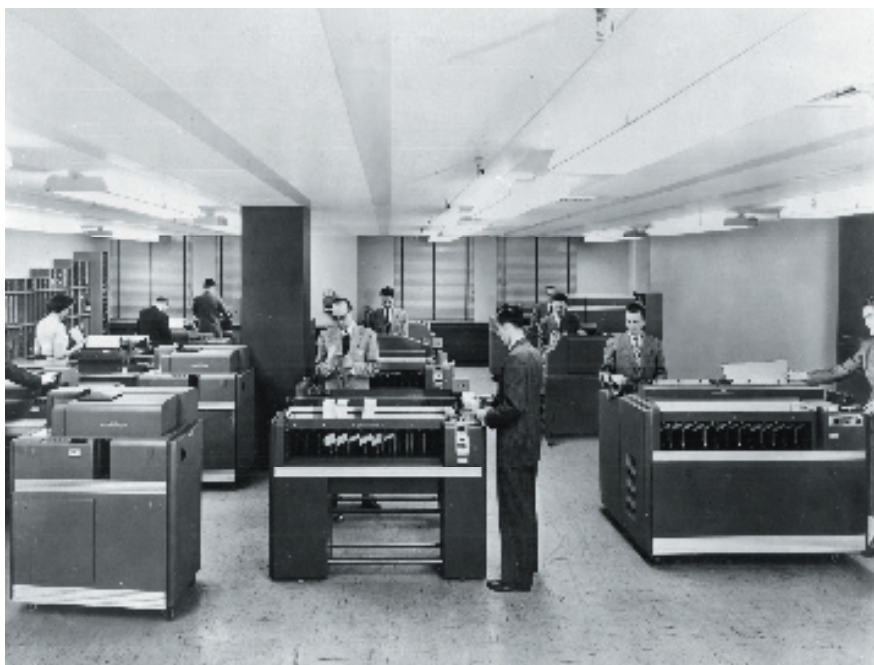
It's 1950 and these 11 men and women are operating an IBM electric accounting machine installation. Seen here (at left) is an IBM 523 gang summary punch, which could process 100 cards a minute and (in the middle) an IBM 82 high-speed sorter, which could process 650 punched cards a minute. (Credit: IBM Archives)
